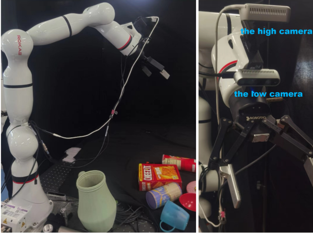
Figure 7. Real-world Handover System Setup. Our system consists of an xMate 3 robot, which is similar to a Franka Panda robot, and two RealSense Depth Camera D435 devices.
